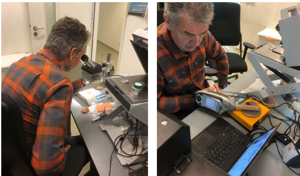
Figure 6.1. The p-XRF in use in the laboratory stand (left) and hand-held (right).
