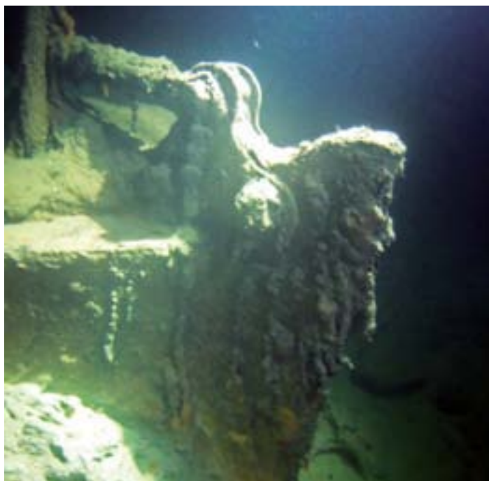
FIGURE 3a-b The intact sternpost of the 90-metre wreck of SS Ingrid Horn is almost covered in sediment. We can also see that the wooden structures are almost entirely intact. Photo: Jakob Selbing
