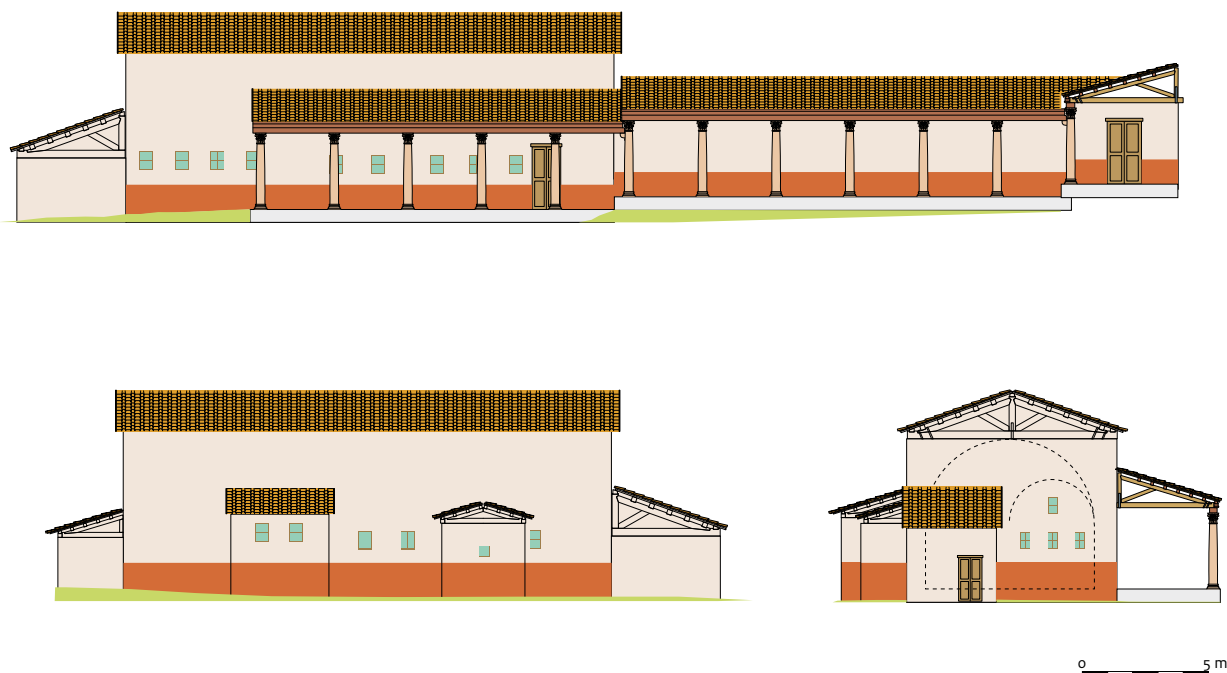
Fig. 8.16 Voerendaal-Ten Hove. Reconstruction of the exterior of the baths with outlines of the roof trusses and in the south façade an indication of the level of the upper hypocaust floor and the top of barrel vaults.
