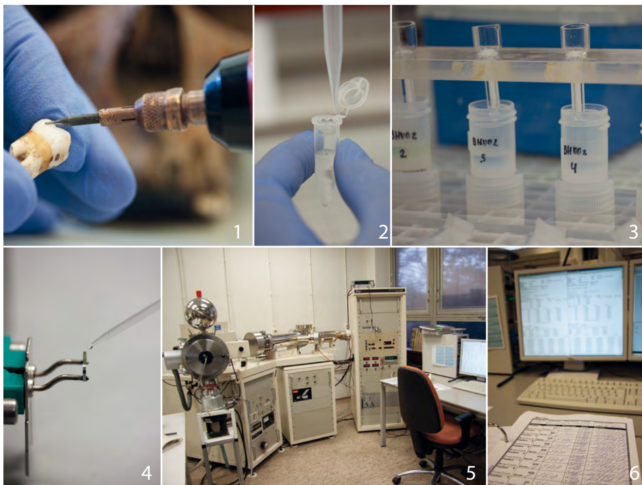
Figure 4.4. Overview of the standard workflow for strontium isotope analysis. Key: 1 – sampling dental enamel; 2 – dissolving the samples in \text{HNO}_3 in a clean laboratory; 3 – strontium extraction/separation by column chromatography; 4 – loading 1 \mu\text{l} of sample on a rhenium filament; 5 – Finnigan MAT 262 TIMS equipment at the Vrije Universiteit Amsterdam; 6 – data collection (photos Lisette M. Kootker).
