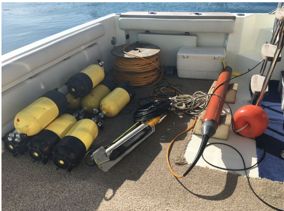
Figure 4 - Side-scan sonar (centre) and magnetometer (right) devices on board the Pilar II.
