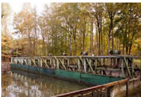
219 This Waterloopbos (Watercourse Forest) model is part of a so-called wave machine used for embankments stability tests.
