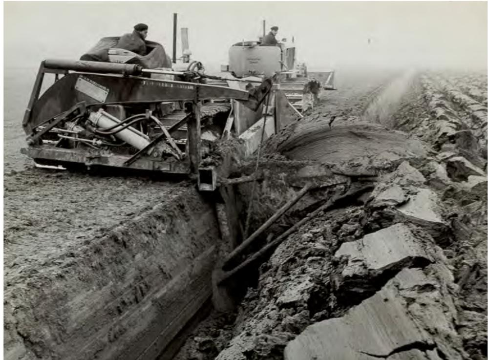
114 Deep ploughing in Noordoost Polder with two ‘Caterpillar machines’ in line drawing the ploughshares. (Exact place and date unknown).
