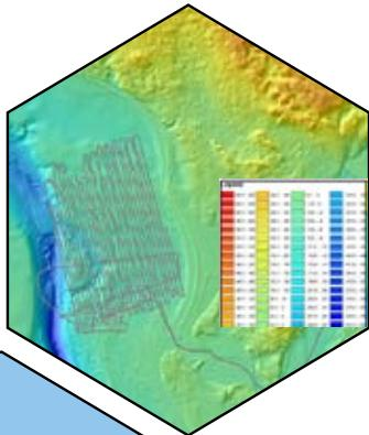
*Seamless map of coastline and seabed generated using a combination of Lidar, and remote sensing techniques including multibeam sonar. Image: GEUS*
