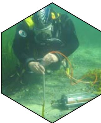
*Diver using a micro sensor to measure environmental parameters under water. Image: Unisense*
