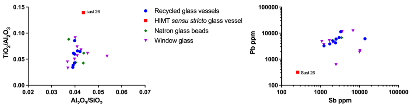
Figure 5.17 Plots of \text{Al}_2\text{O}_3/\text{SiO}_2 against \text{TiO}_2/\text{Al}_2\text{O}_3 (a) and Sb against Pb (b) for Susteren natron glass samples.
